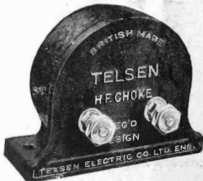
TELSEN H.F. CHOKES. Designed to cover the whole wave-band range from 18 to 4,000 metres, extremely low self-capacity, shrouded in Genuine Bakelite. Inductance 150,000 henries. Resistance 400 ohms. Price 2/6 each.
