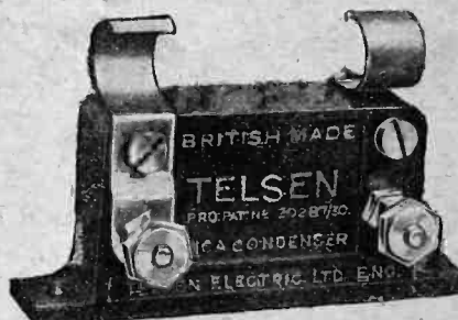
TELSEN FIXED (MICA) CONDENSERS. Shrouded in Genuine Bakelite, made in capacities up to .002 mfd. Pro. Pat. No. 20287/30. .0003 supplied complete with Patent Grid Leak Clips to facilitate series or parallel connection. Can be mounted upright or flat. Tested on 500 volts. Price 1.- each.
